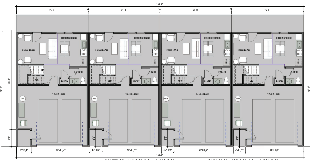
1 FULL MAIN LEVEL HEATED SF - 460.8 SF X 4 = 1,843.2 SF GARAGE SF - 499.2 SF X 4 = 1,996.8 SF
